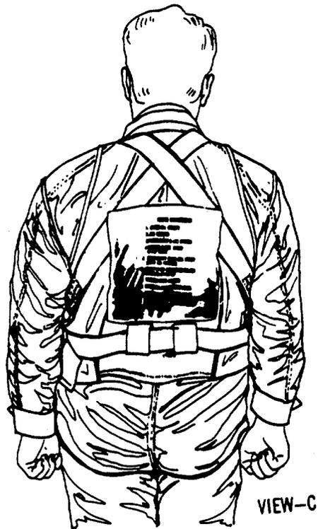
Figure 1-4. Adjustable Parachute Ejection Seat Restraint Harness for OV-1 Mohawk.
