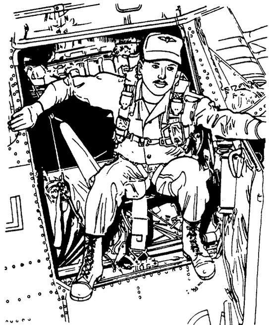
Figure 2-12. Pilot Bailout Door Position From O-A1 and TO-1A. Typical
