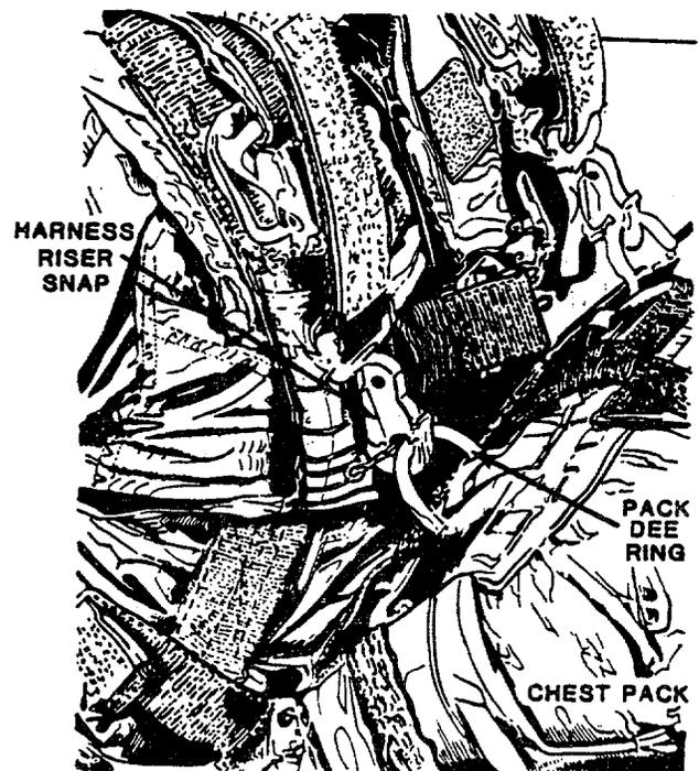
Figure 2-9. Attaching Chest Pack to Harness Assembly.
