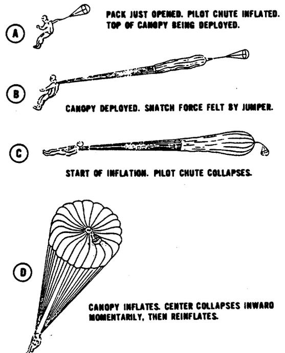
**Figure 2-14. Deployment and Inflation of a Parachute Canopy.**
