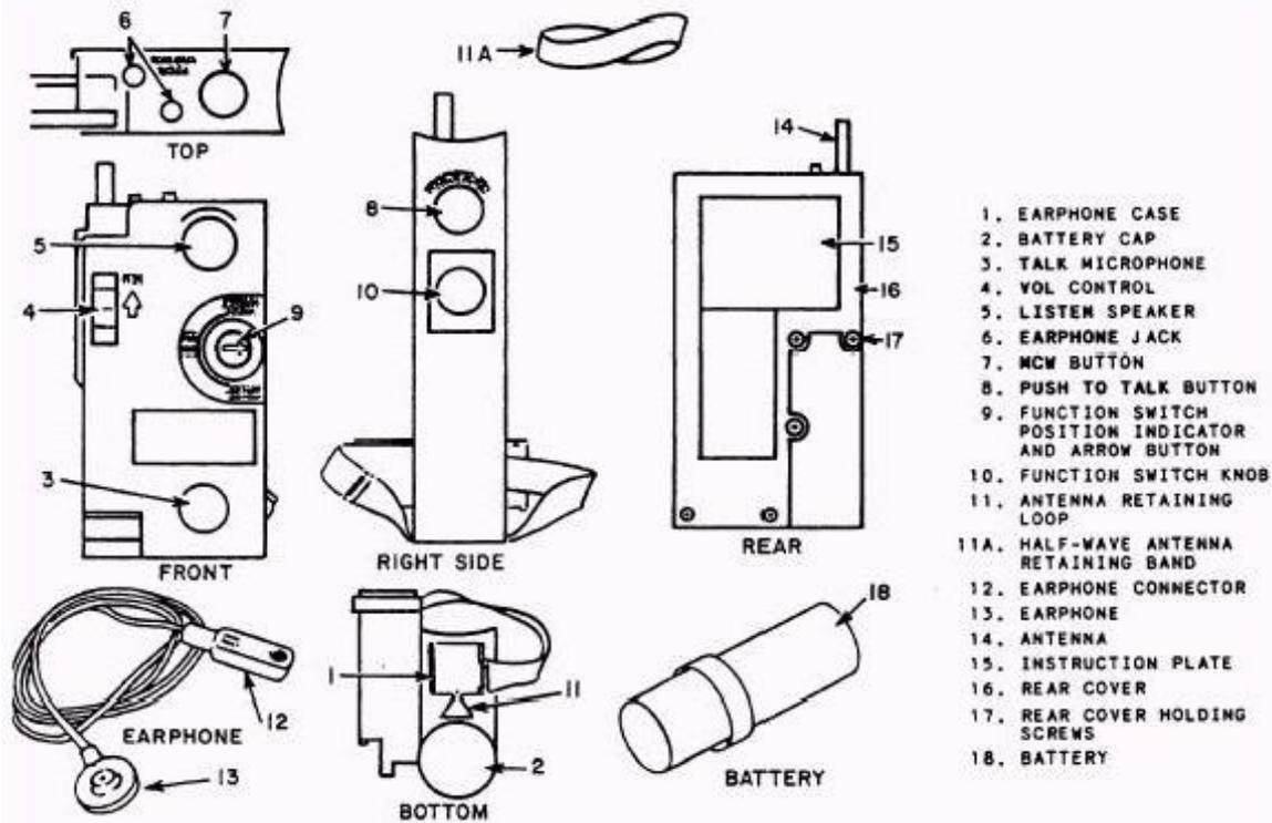
Figure 5-8.-AN/PRC-90 controls and indicators.
